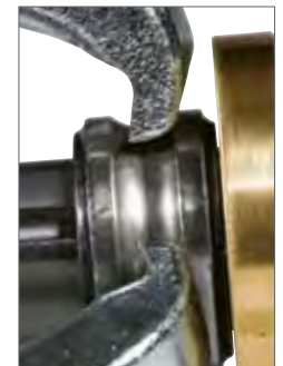
Lock on ball grooves and bearing races.
