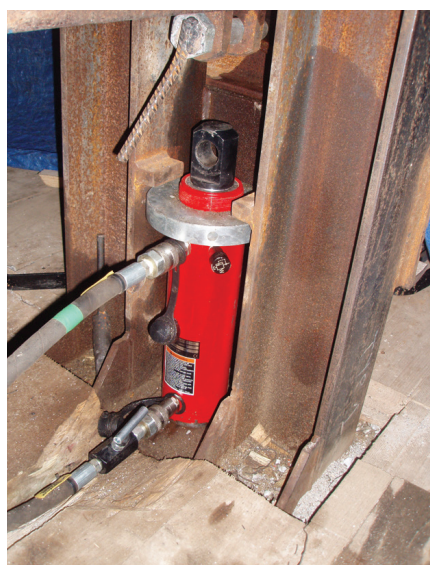
HD cylinders can be used in pushing and pulling applications. In this photo, we see a HD2506 HD cylinder set up for a pull application using a rod clevis cylinder accessory
