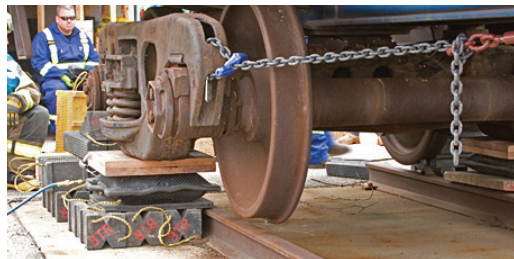
A lifting bag raising the axle of this train car for maintenance
